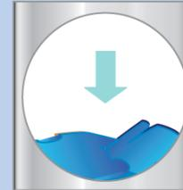
The machine is pressurized. CO<sub>2</sub> turns from a gas to a liquid under pressure.
